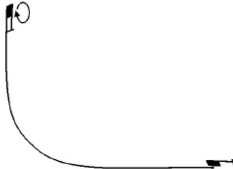
**5. Slow Roll.** Model flies straight and level for a minimum of 10m, rolls through one (1) complete 360 degree revolution maintaining the nose in the direction of flight, flies straight and level for the same duration and at the same altitude as the entry. Manoeuvre is centred with the model inverted at the midline and the roll portion of the manoeuvre should have a duration of 3 seconds minimum.
