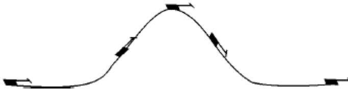
**7.Approach and Go Around (downwind).** At an altitude of no less than 10m and on a heading parallel to the flight line, the helicopter begins a constant rate descent and deceleration to be stopped above the central helipad, pause, climb and accelerate to a height of no less than 10m. The descent and climb paths should be approximately 45 deg and symmetrical to each other. This manoeuvre must be done in the opposite direction to manoeuvre 8. This is to demonstrate approaches from both sides.
