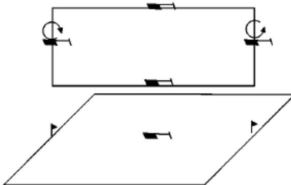
**4. 540 Degree Stall Turn.** Model flies straight and level for 10m then climbs with a smoothly-rounded curve of 90 degrees to a vertical climb. When the vertical climb stops, the model rotates 540 degrees about the yaw axis so that the nose points downward. While diving, the model
