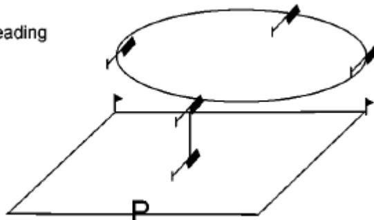
**3. Tail-in Vertical Rectangle.** Model takes off from the central helipad and rises vertically to eye level, pauses, maintaining a constant altitude, heading, and speed, hovers sideways either direction, to the edge of the box, pauses, rises vertically 2m, pauses, hovers sideways over the central helipad to the opposite side of the box, pauses, descends vertically 2m, pauses, hovers back to central helipad, pauses, and descends vertically to the central helipad.
